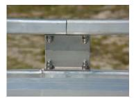
and half on the side rail - position the join in the middle. Position the front one midway between the rear and the front of the side rail. Mount the side rail on top of these plates, bolting the front down with the one bolt you left right in the front of the rack. Tighten all in place(keep loose for minor adjustment), repeat for back rail and other side rail.
